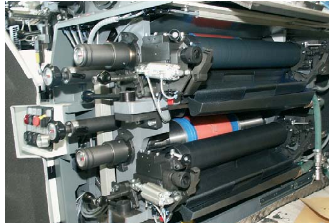
Flexo printing unit for outside printing
