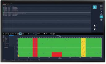
**Defender Waste Manager** can interface to rewinding, slitting, and sheeting equipment to automatically control when they stop/reject—allowing for fast and easy removal of defective material.
