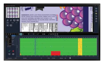
**Defender Data Central** uses visual maps of each inspected roll so quality control operators can analyze for defect distribution, count, and type. Out-of-tolerance areas are identified for removal, and job-based quality reports can be generated.
