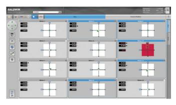
Ribbon Control with MultiCam displays all ribbons at a glance, and the system automatically keeps your print run within established tolerances.
