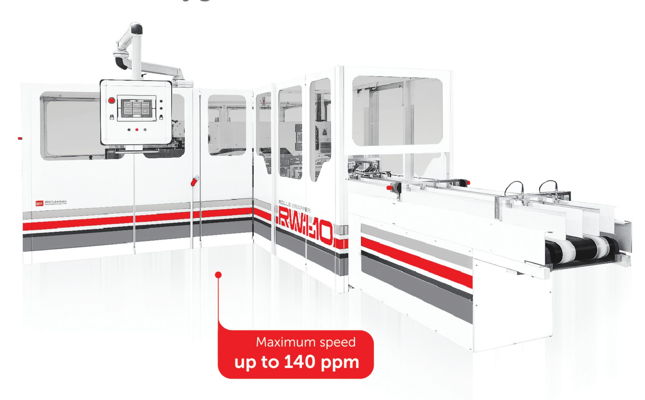
The **RW1-10** wrapper is a packaging machine for hygienic and kitchen rolls very economical and efficient. It packs from 1 to 12 rolls, with single layer, and also 1 and 2 kitchen towels. This wrapper is easy to use, it is fully servo driven, controlled by the most advance motion controller OMRON - NJ501 which allows extremely quick format changeover. It reaches output production speed up to 140 packs/minute.
