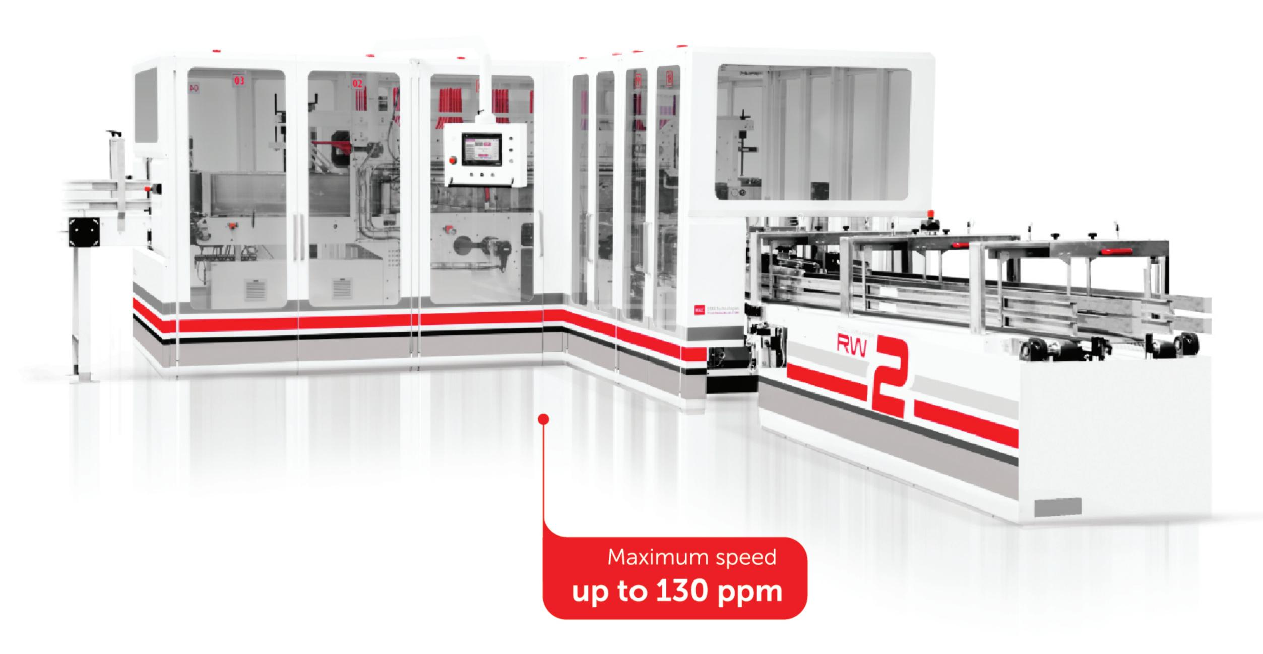
The RW2-AFH wrapper is a packaging machine for industrial rolls, very economical and efficient. It packs from single roll to 2 rolls in a row, a single layer, with 2 lanes infeed, with a production speed up to 130 packs/minute.
