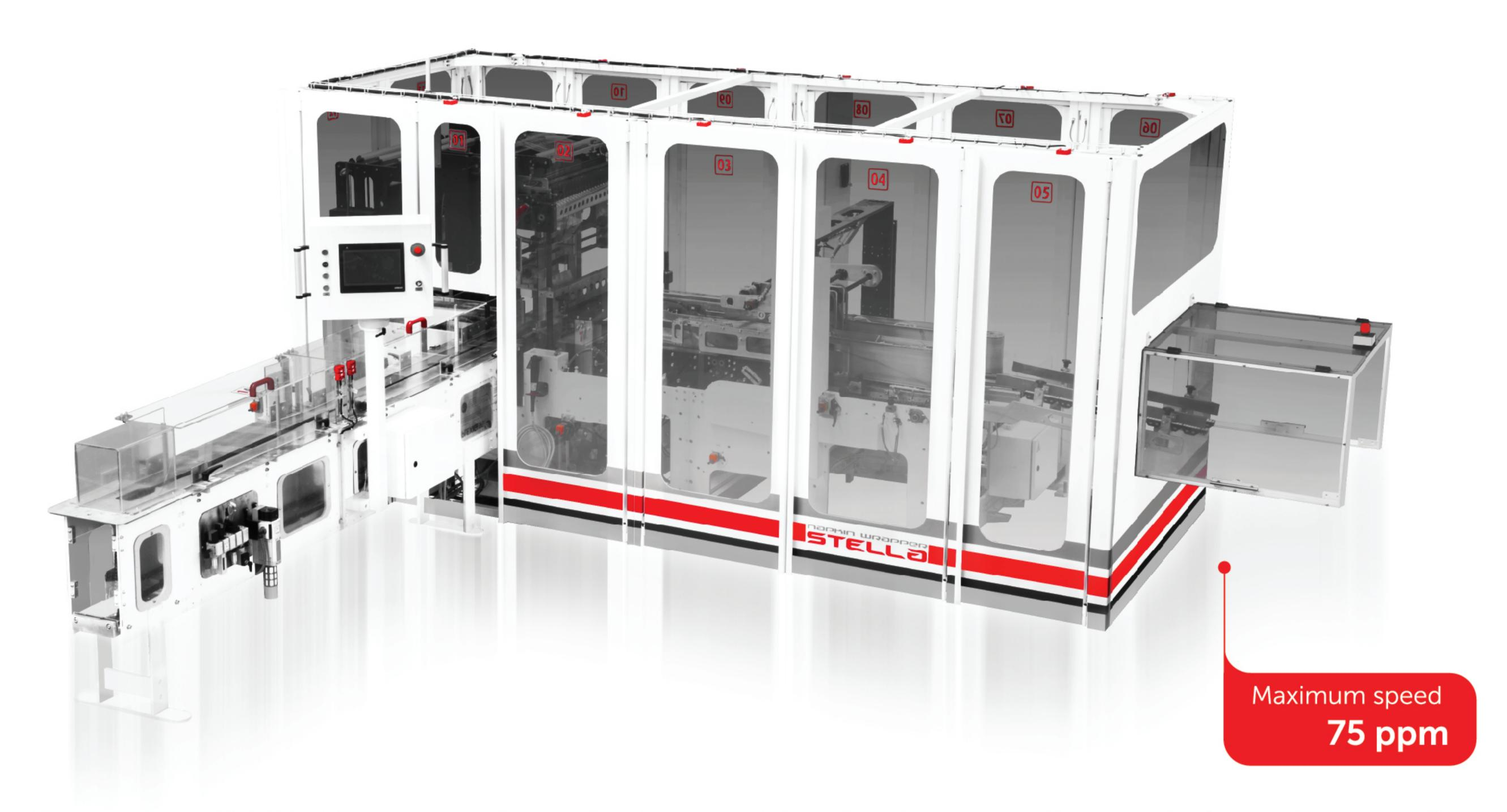
Napkin wrapper **STELLA** is automatic packaging machine for tissue napkins, folded towels, as well as non-woven folded products. This is our flagship napkin wrapper, very economical and efficient. It can pack up to 75 single packs and up to 50 double packs with max width of 440 mm (17.3").
