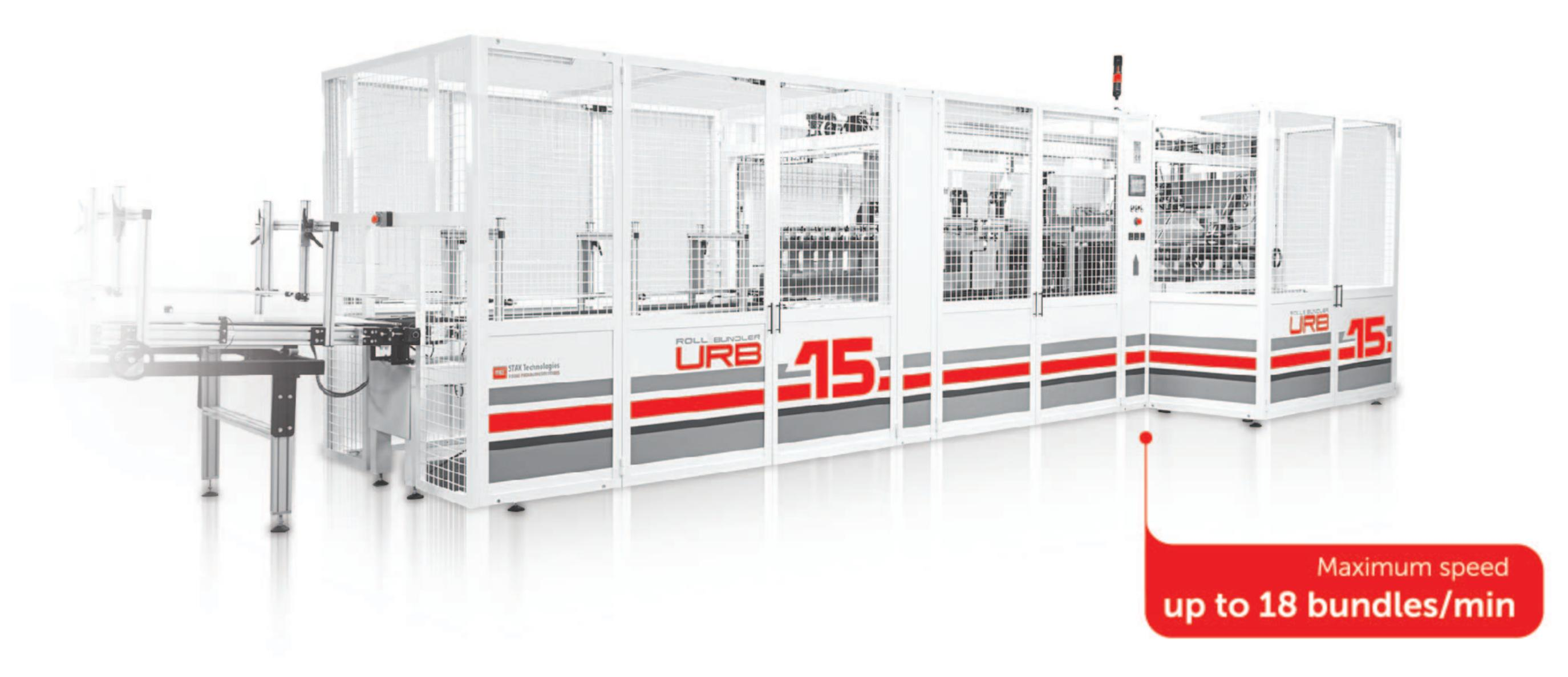
Universal Roll Bundler **URB-15** is flexible high-speed bundling machine for grouping and over-wrapping different configurations of bathroom tissue and household towel roll packs with horizontal and vertical cores.
